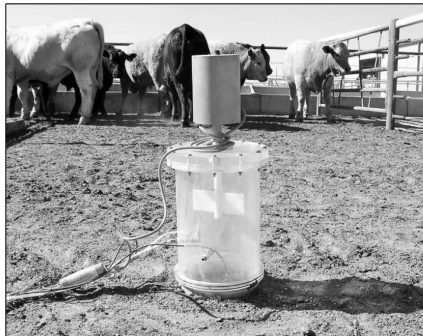
Figure 3. A portable dynamic flow-through chamber was used for measuring ammonia flux from the beef feedyard pen surface.
