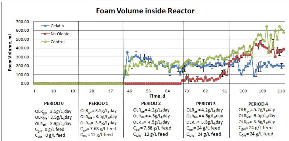
Fig. 7 Foam formation in the biogas reactors fed with manure supplemented with protein, or lipid, or carbohydrate
