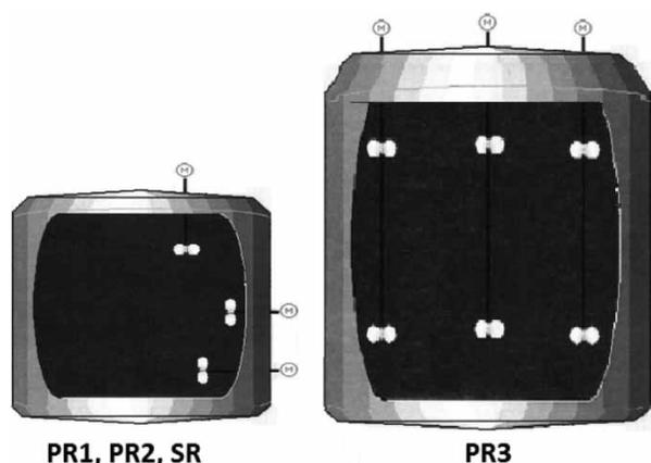
Figure 3 | Stirring pattern of biogas reactors at Lemvig biogas plant.
