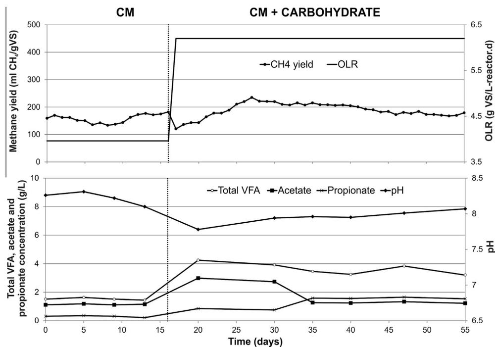
Fig. 6. Process performance of reactor (R3) fed with CM and glucose (carbohydrate).
