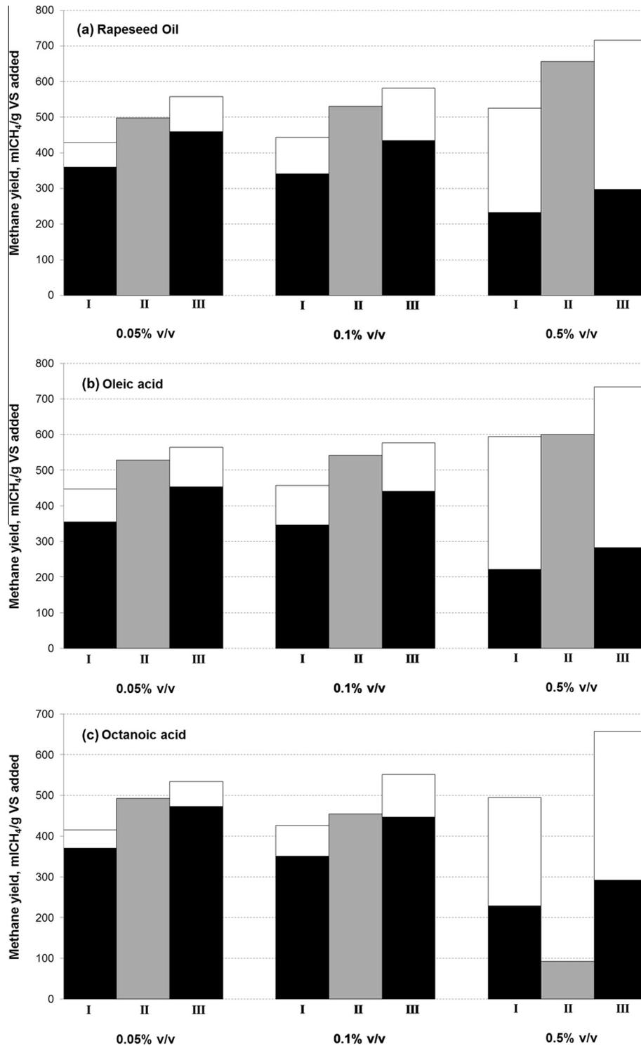
**Fig. 1.** Methane yield of cattle manure (black column), antifoams (white column), and mixture of cattle manure with 0.05%, 0.1% and 0.5% v/v antifoams (grey column); (I) from BMP assays of single substrates, (II) from BMP assays of mixed substrates, and (III) from theoretical yield.
