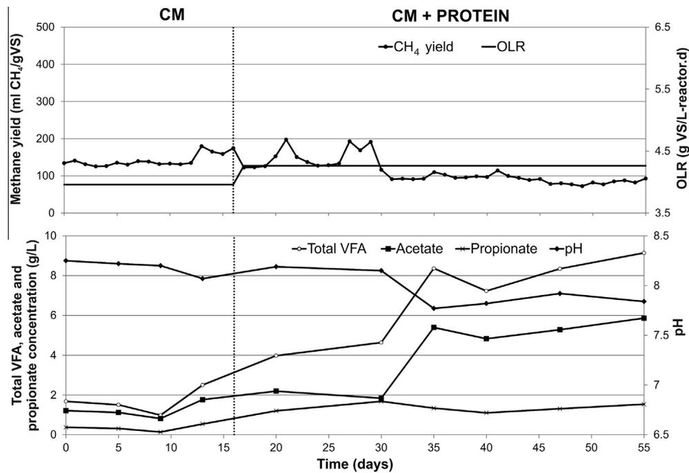
**Fig. 4.** Process performance of reactor (R1) fed with CM and gelatin (protein).
