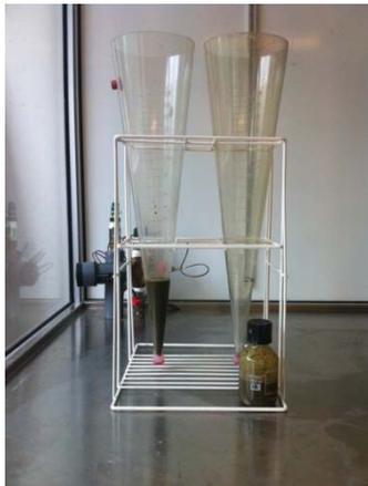
**Fig. 4** Apparatus used for the determination of foaming tendency and stability
