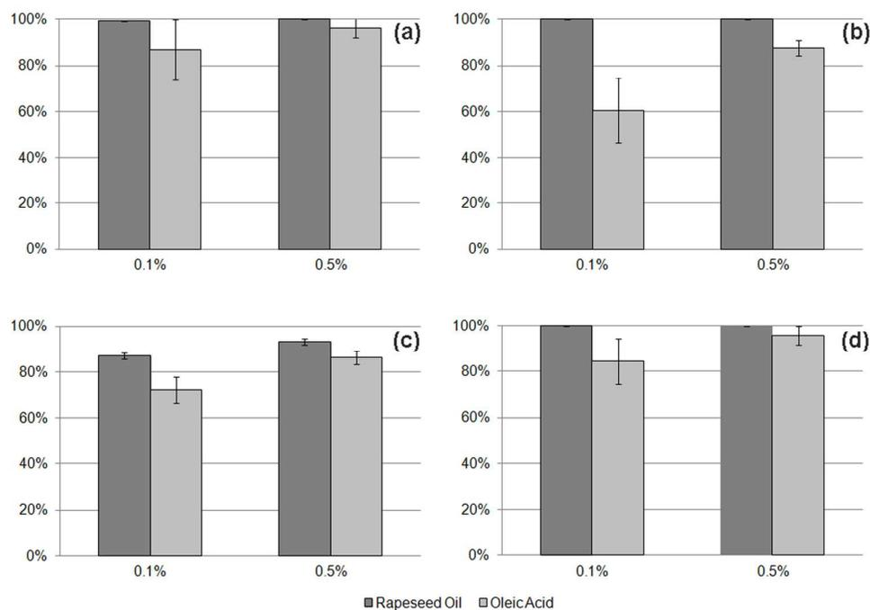
Figure 1. Defoaming efficiency (%) of rapeseed oil and oleic acid in (a) raw cattle manure, (b) digested cattle manure supplemented with proteins, (c) digested cattle manure supplemented with lipids, (d) digested cattle manure supplemented with carbohydrates. Both defoamers were tested at concentrations of 0.1% v/vsample and 0.5% v/vsample.
