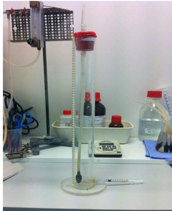
**Fig. 9** Bottom injection method; the antifoam is directly added in the manure sample.
