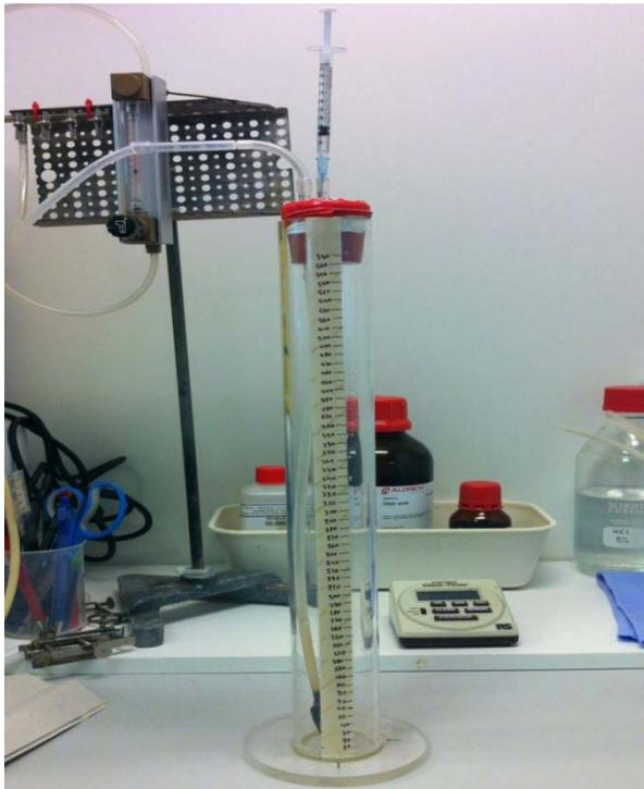
**Fig. 8** Headspace injection method; the antifoam is sprinkled from the top of the aeration column.
