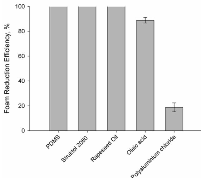
Figure 2. Foam reduction efficiency of chemical agents.
