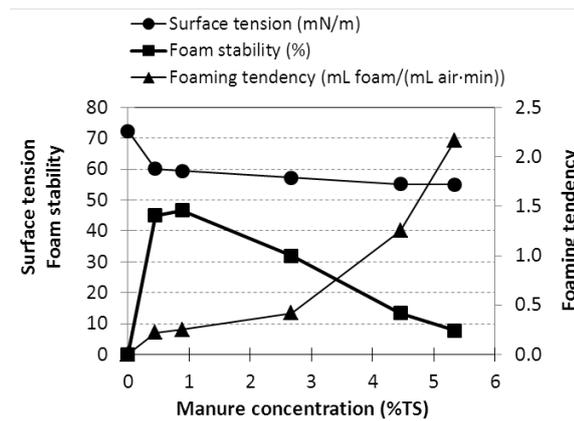
**Fig. 5** Surface tension and foaming potential of manure at different concentrations
