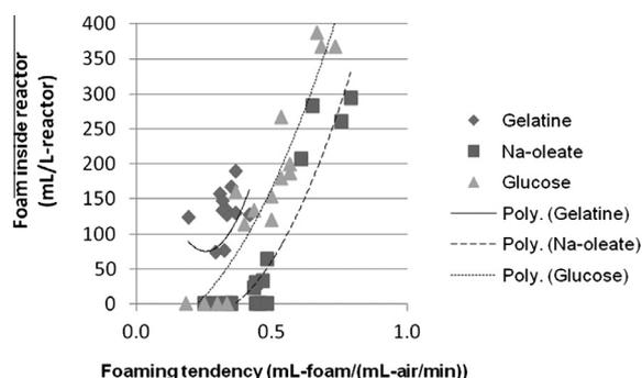
Fig. 5. Correlation of foaming tendency and the volume of foam produced inside the reactors.
