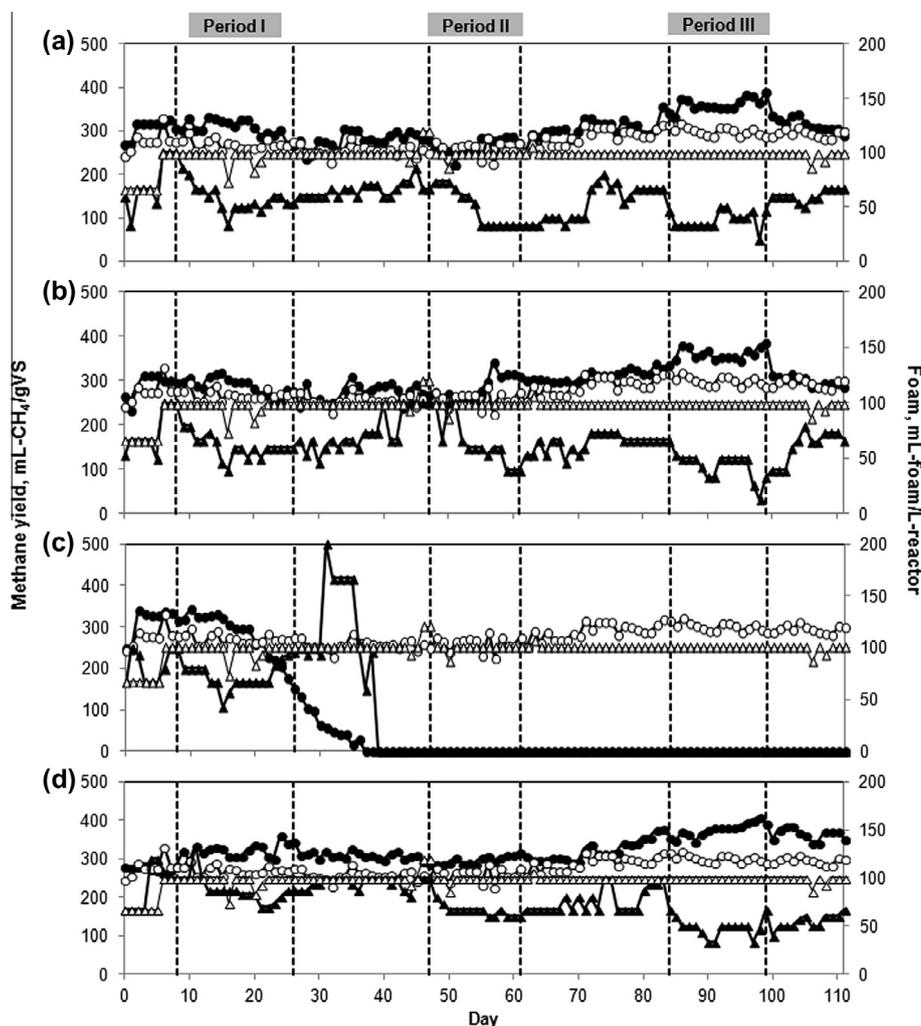
**Fig. 2.** Methane yield and foam formation in the control reactor (○ and △, respectively), compared with the reactors treated with rapeseed oil (a), oleic acid (b), tributylphosphate (c) and octanoic acid (d). Periods (I), (II) and (III) corresponded to antifoam dosages of 0.05%, 0.1% and 0.5% v/v<sub>feed</sub>, respectively. Symbols ● and ▲ represent methane yield and foam formation in the treated reactors, respectively.
