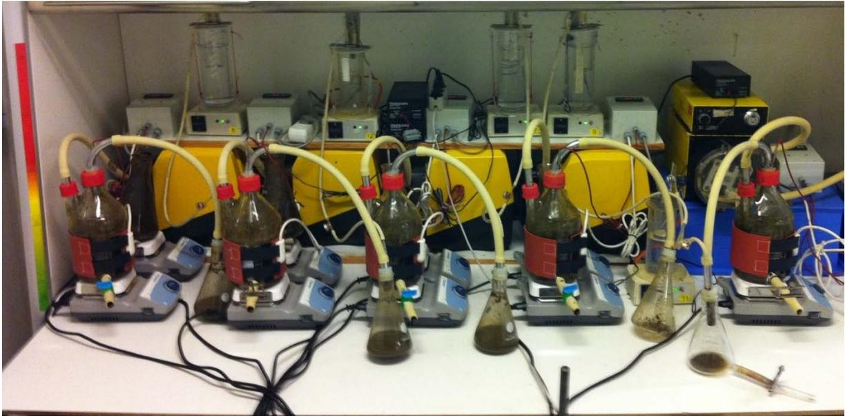
Fig. 6 Experimental setup of continuously fed biogas reactors
