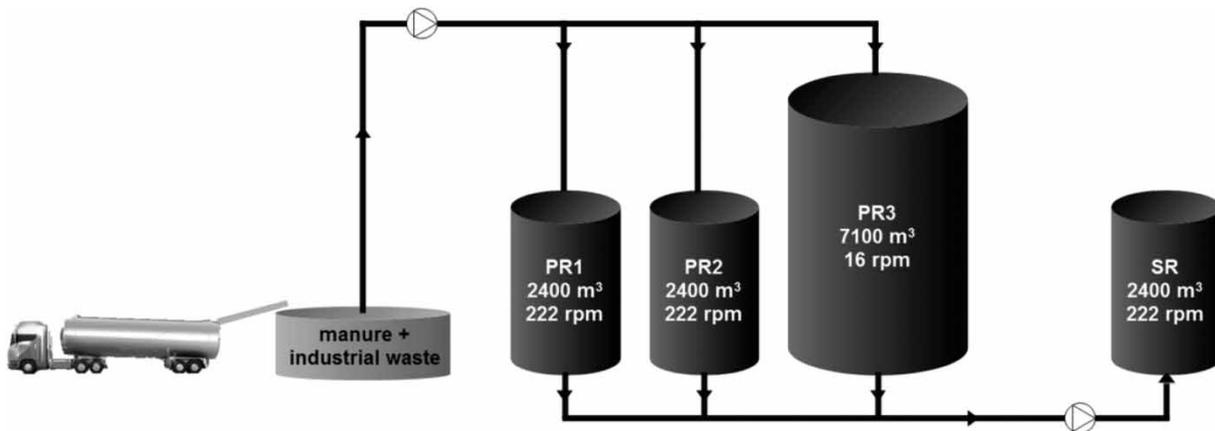
Figure 2 | Lemvig biogas plant reactors scheme.
