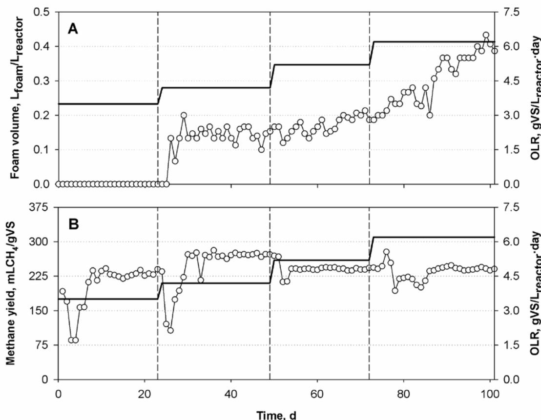
Figure 1. Correlation of OLR with A) foam volume inside the reactor, B) methane yield.
