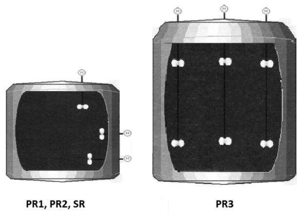
**Fig. 3** Stirring pattern of biogas reactors at Lemvig biogas plant. PR3 is the foaming reactor.
