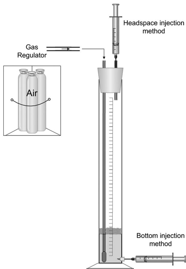
**Fig. 1 – Foaming apparatus used for the aeration method.**
