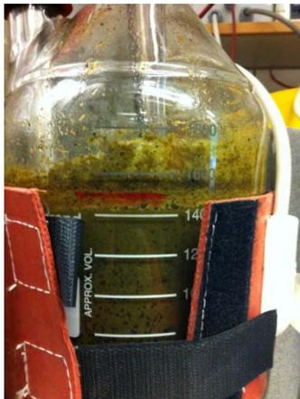
**Fig. 10** Foam formation in CSTR overloaded with carbohydrate-rich manure substrate.
