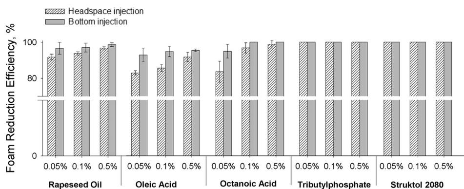
Fig. 4 – Foam reduction efficiency of antifoaming agents during headspace and bottom injection methods.
