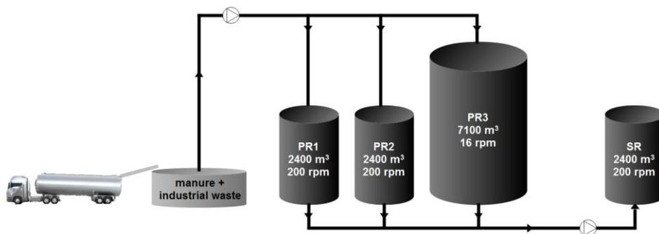
**Figure 2.** Lemvig biogas plant reactors.
