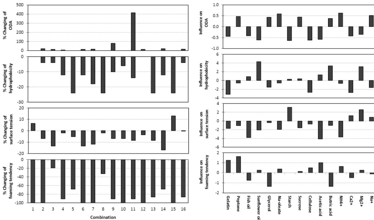
**Figure 3.** Effect of substrates and intermediate compounds in a complex mixture; a) Change of liquid properties and foaming potential in manure solution with different combinations of compounds, b) Statistical analysis for the influence of compounds on liquid properties and foaming in the manure mixture
