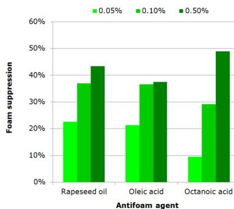
**Fig. 11** Foam suppression efficiency of the tested antifoaming agents.
