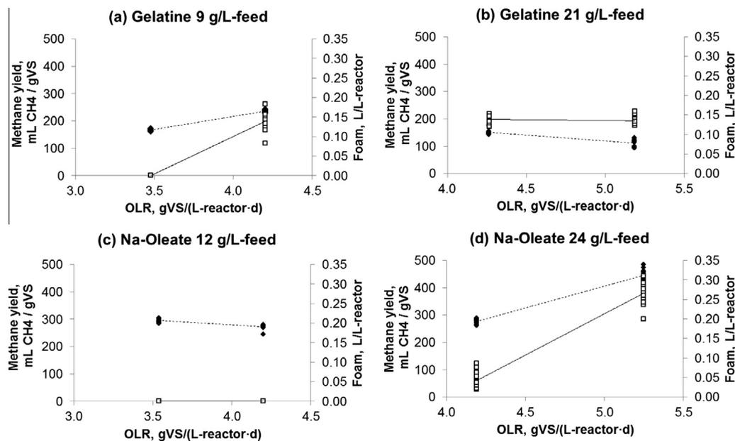
Fig. 2. Effect of OLR on methane yield (◆) and foam formation (□) with the addition of gelatine or Na-Oleate, or glucose.
