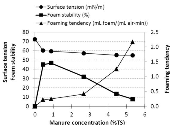
**Figure 2.** Surface tension and foaming potential of manure at different concentrations
