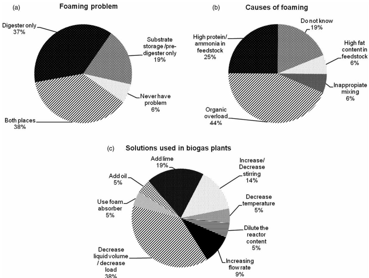
**Figure 1** | Results from survey for the Danish full-scale biogas plants: (a) occurrence of foaming incidents, (b) potential causes of foaming, and (c) solutions applied to suppress foaming.
