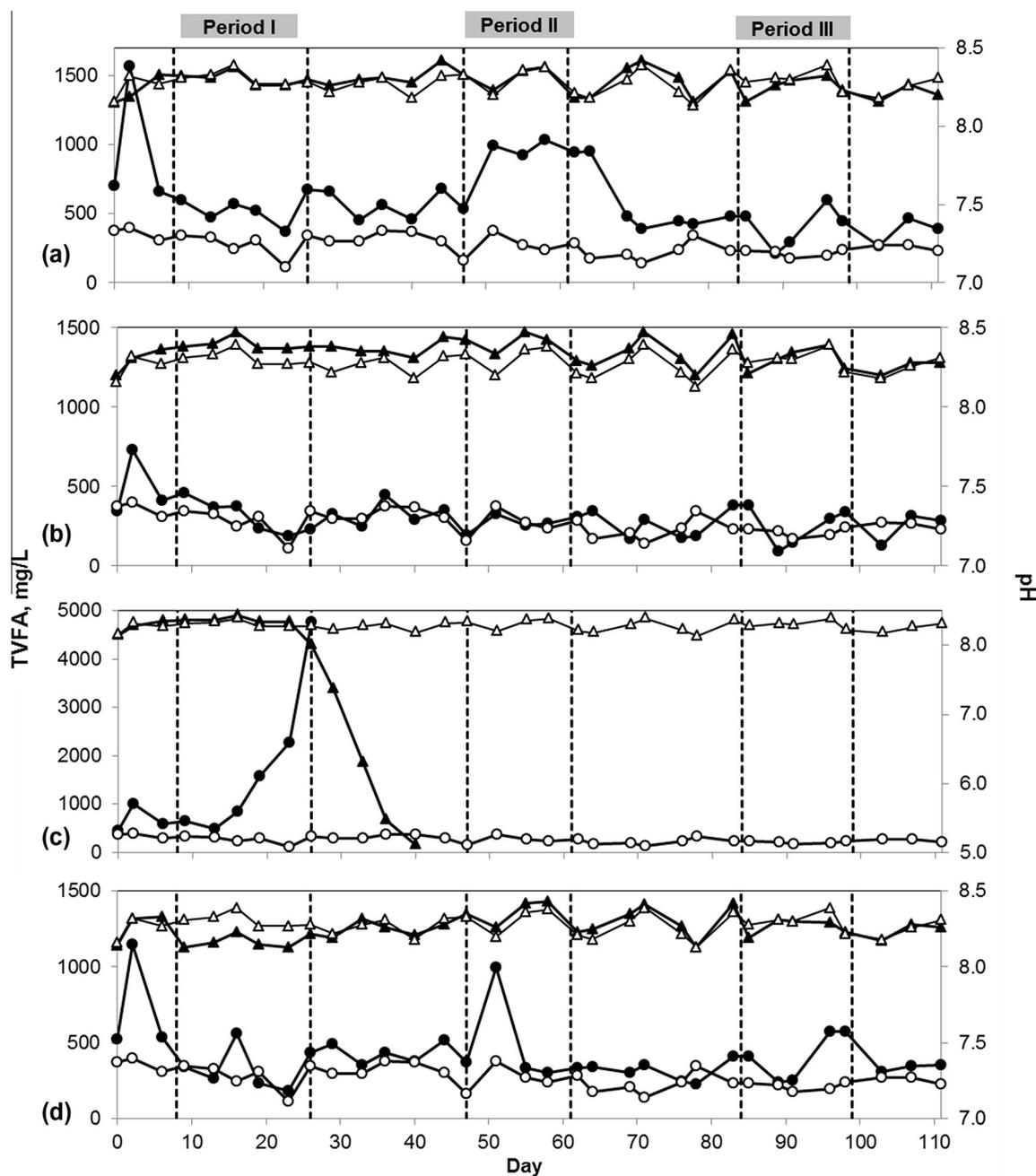
**Fig. 3.** Total volatile fatty acids (TVFA) and pH in the control reactor ( $\circ$  and  $\triangle$ , respectively), compared with the reactors treated with rapeseed oil (a), oleic acid (b), Tributylphosphate (c) and Octanoic acid (d). Period I, II and III corresponded to antifoam dosages of 0.05%, 0.1% and 0.5%  $v/v_{\text{feed}}$ , respectively. Symbols  $\bullet$  and  $\blacktriangle$  represent TVFA and pH in the treated reactors, respectively.
