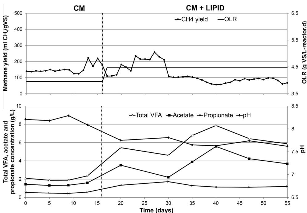
Fig. 5. Process performance of reactor (R2) fed with CM and Na-Oleate (lipid).
