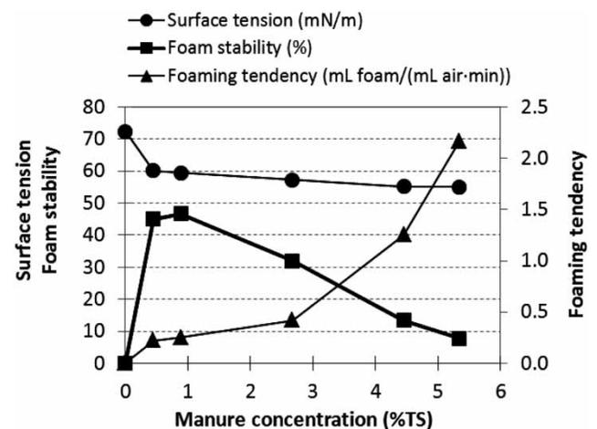
Figure 2 | Surface tension and foaming potential of manure at different concentrations.
