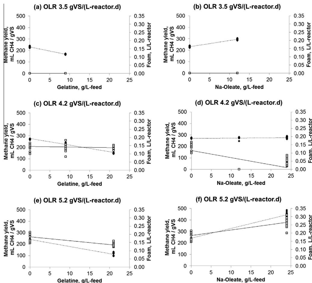
Fig. 4. Effect of protein (a, c, e) and lipid (b, d, f) on methane yield (◆) and foam formation (□) Na-Oleate at OLR of 3.5 (a, b), 4.2 (c, d), and 5.2 (e, f) gVS/(L-reactor-day).
