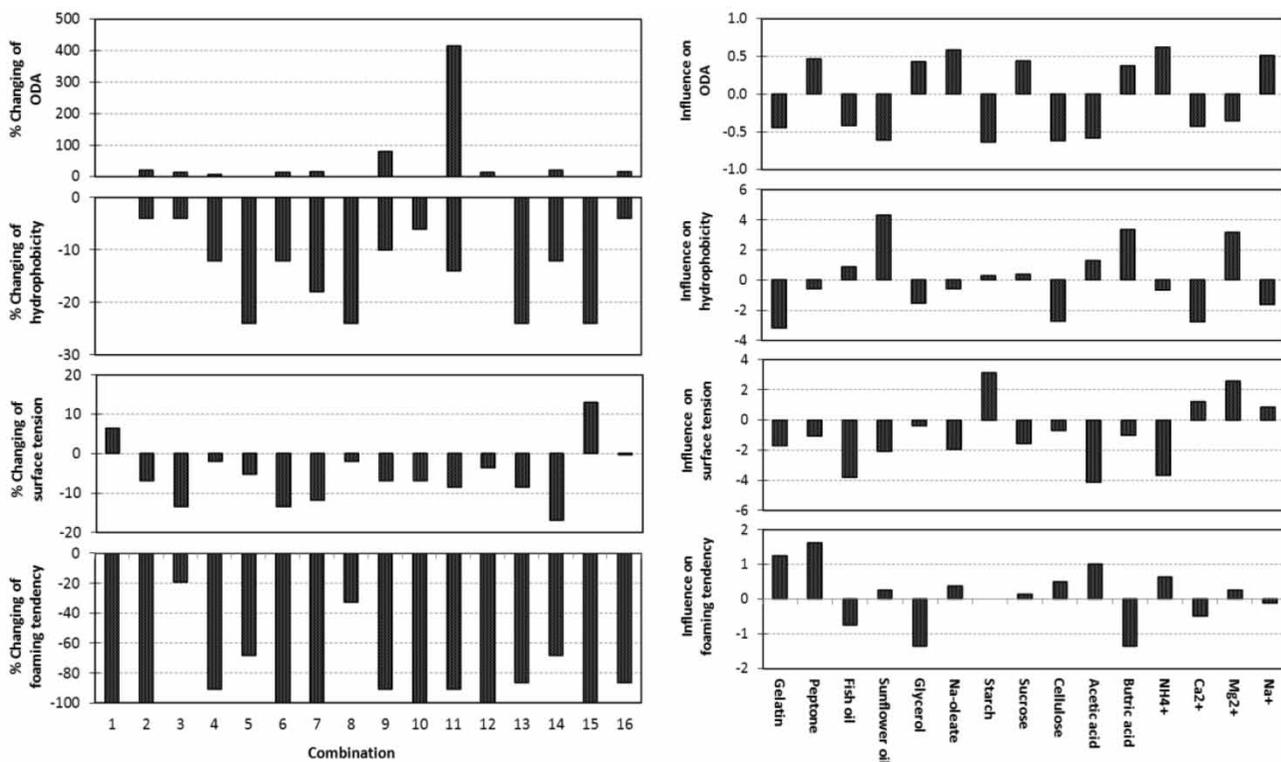
Figure 3 | Effect of substrates and intermediate compounds in a complex mixture; (a) change of liquid properties and foaming potential in a manure solution with different combinations of compounds, (b) statistical analysis for the influence of compounds on liquid properties and foaming in the manure mixture.
