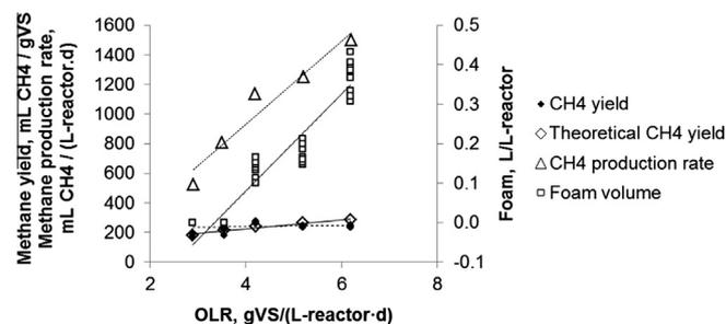
**Fig. 1.** Effect of OLR on methane yield, methane production rate, and foam formation without addition of protein or lipid. The OLR was increased by adding glucose.
