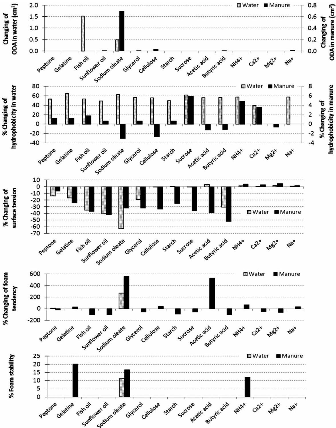
Figure 1 | Effect of feedstock compounds on solution properties and foaming in water and manure.
