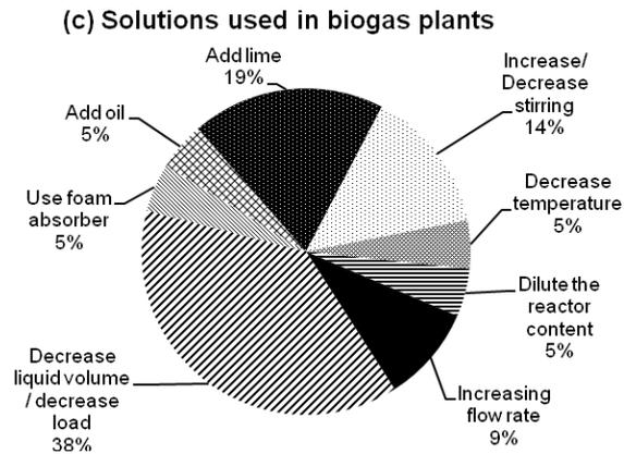
**Figure 1.** Survey for the (a) occurrence of foaming incidents, (b) causes of foaming and (c) solutions used to suppress foaming in Danish full-scale biogas plants.
