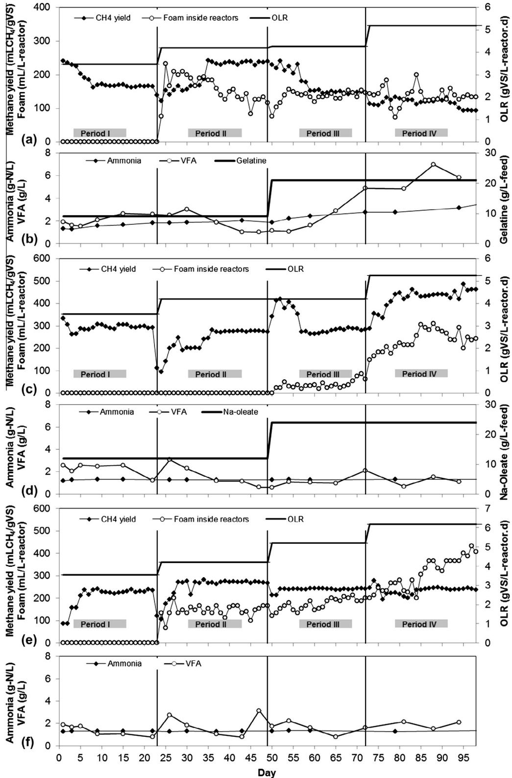
Fig. 3. Process performance of reactor R1&R2 (a, b), R3&R4 (c, d), and R5 (e, f) during all periods of experiment.
