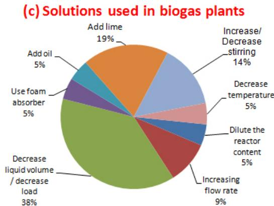
**Fig. 1** Results from survey for the Danish full-scale biogas plants; (a) occurrence of foaming incidents, (b) potential causes of foaming, and (c) solutions applied to suppress foaming
